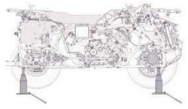
Schematic diagram of jack support position
