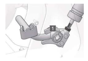
The foot brake lever adjusting nut is located at the bottom of the vehicle near the foot brake lever. The stroke height of the foot brake lever can be adjusted by twisting the foot brake lever nut.
