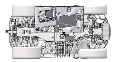
1 Bolt 2 Filter inspection cover 3 Oil drain plug 4 Gasket
