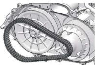
4. with the kit-out pin for driven pulley(special tool) against the driven wheel as shown in the figure of the hole, make the driven wheel open.
