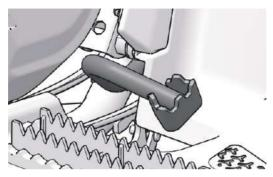
The foot brake is the main brake system of the vehicle. The main brake is located on the right foot plate of the vehicle. When the vehicle needs to slow down or stop, step on the foot brake slowly. Emergency braking can cause the vehicle to skid or roll over, so do not use emergency braking when it is not necessary.
