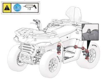
These parts in the vehicle needs sufficient lubrication, according to the maintenance of the periodic table to add appropriate grease. lubrication, can reduce the wear of these parts, and increase the service life
