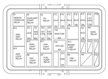
Rated amperage of fuse/relay and distribution
