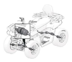
Check the front and rear drive shaft boots for cuts, cracks. damage or grease leaks. If so, contact your Segway dealer for a replacement.
